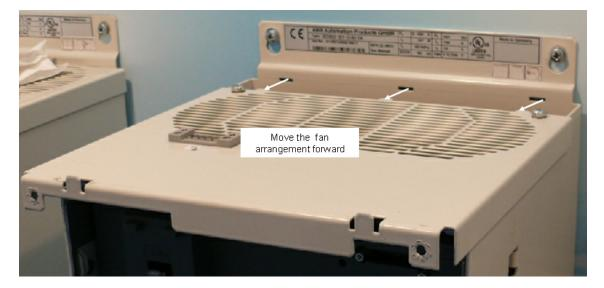
4. Remove the fan holding screws:
