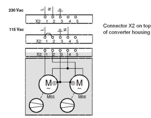
In case a fan fails there are different approaches due to the incoming voltage.
