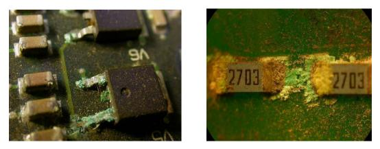
A harsh environment, such as high ambient temperature, humidity, dust and cyclic heavy load, not only shortens the components lifetime but also the preventive maintenance and replacement intervals.
