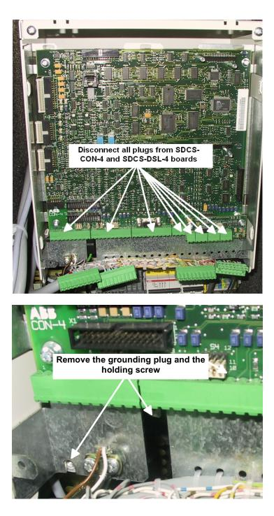
5. Remove the grounding plug and the holding screw at the electronic tray
