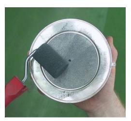
4. Centre the thyristors by means of the spring pins. **Note:**
