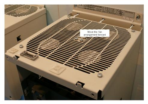
4. Remove the fan holding screws:
