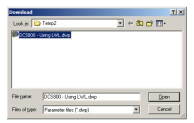
To check, if the parameter download was successful, connect the drive with DriveWindow and compare the drive memory with the downloaded parameter set. Click *File* then *Parameters* and *Compare...*
