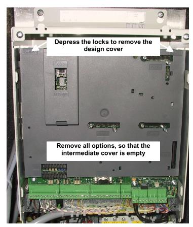
4. Disconnect all I/O plugs (X3 to X7) at the SDCS-CON-4 and the plugs at the SDCS-DSL-4 board, if used (X51 to X54)
