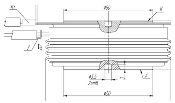
Gate (y): Cathode (K1): Conductive plate: Round terminal D = 1.5 mm Faston 4.8 x 0.5 mm Diameter 50 mm
