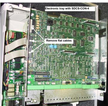
8. Remove all cables and plugs at the SDCS-PIN-4
