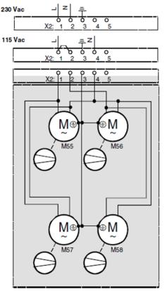
Connector X2 on top of converter housing
