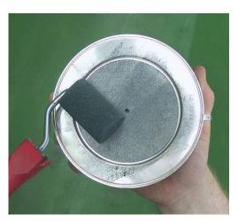
4. Centre the thyristors by means of the spring pins. **Note:**
