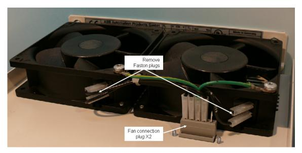
6. Reassemble everything and check for correct blow direction of each fan. The air should be sucked out of the module
