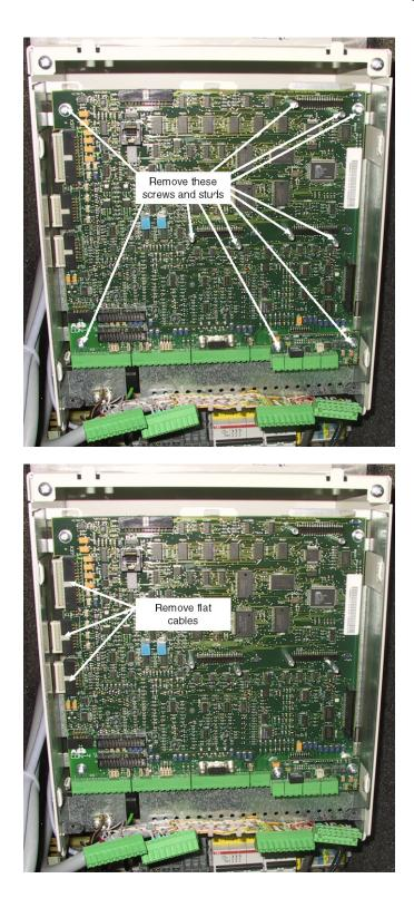
6. Unplug the flat cables (X12, X13, X37)7. Remove the SDCS-CON-4
